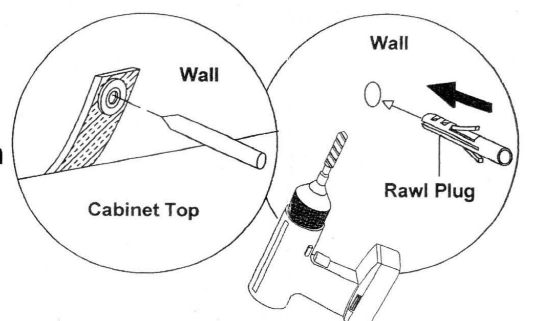
Drill a hole in the wall and insert the rawl plug.
