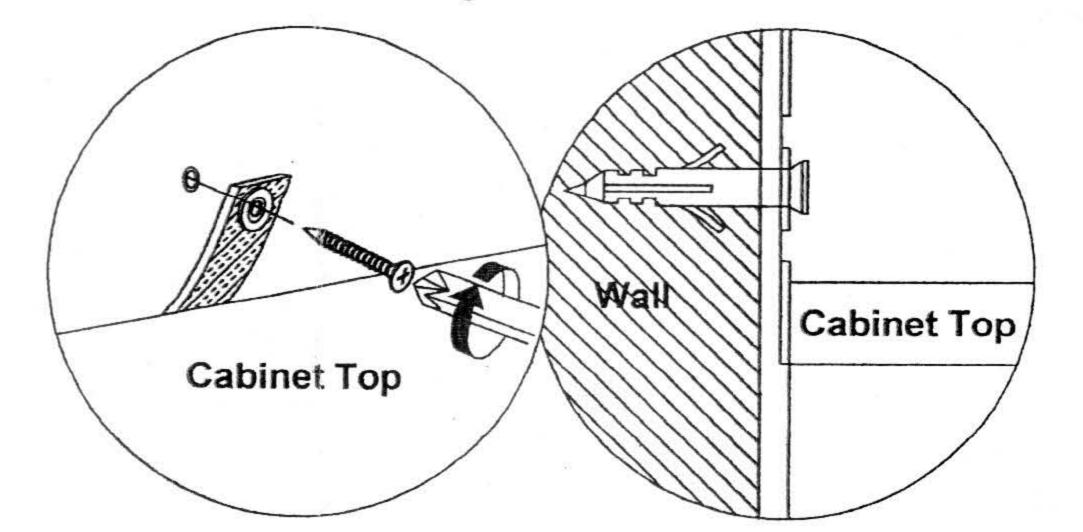
NOTE: Wall fixings are not supplied with this product as different wall materials require different types of fixing devices (such as Rawl plugs on brick work). You must use fixing devices suitable for the type of wall you intend to mount this product to. Please ensure that the head of any screw used as a diameter greater that the diameter of the mounting hole on the bracket and that the fixing is safe and secure before use.
